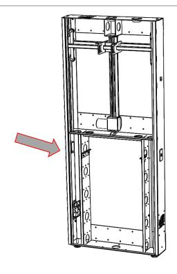
Plug in and test run unit up and down.
